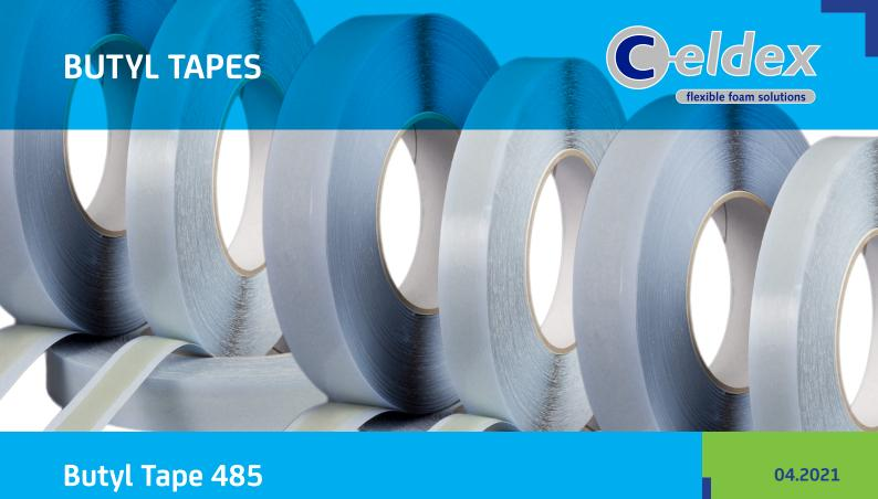
Celdex Butyl Tape 485 is a strip glue, based on butyl rubber and resin. Butyl Tape 485 is suitable as an mounting aid for many construction materials and for the connection of foils and is not UV-resistant. Available on roll in flat shape, in the colour amber.
