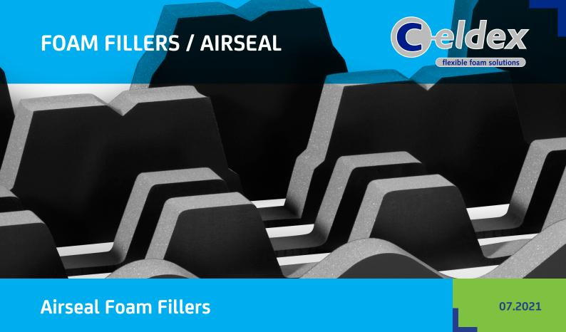
Celdex Airseal Foam Fillers are made from semi-closed-cell polyurethane foam (fitted with a TPU top layer on both sides), custom made, profiled sealing products. The products are applied as durable sealing in profiled steel roof and wall constructions or other applications that require customisation. Airseal Foam Fillers provide protection against draught, heat loss and noise.
