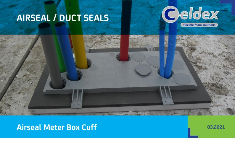
Celdex Airseal Meter Box Cuff is a specially developed sealing cuff that can be used as an airtight layer for the utilities in the meter box. The sealing cuff complies with the strictest requirements for energy-efficient construction and is available for all brands and designs of meter box floor slabs.
