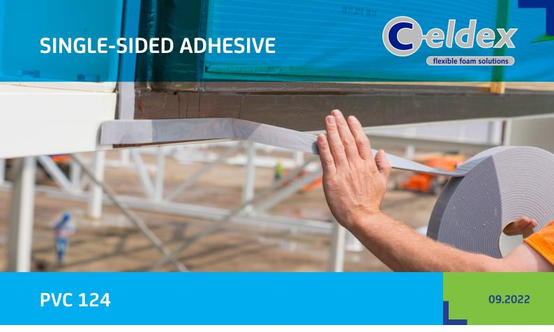
Celdex PVC 124 is a soft semi-closed-cell PVC foam. The top side of the foam tape is fitted with a low friction mylar foil. Suitable as an airtight sealing for parallel surfaces. The tape must be sufficiently compressed in order to meet specifications, such as airtightness, thermal and acoustic insulation.
